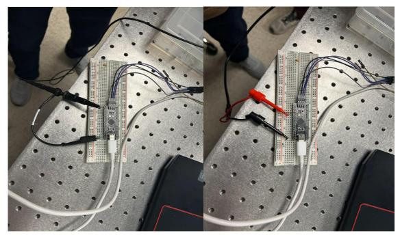
The above two images are the working circuit with connection to a DC voltage supply and then moving onto the AC voltage supply. This circuit was used for the DMA ADC, the one we are currently working to fine tune.
